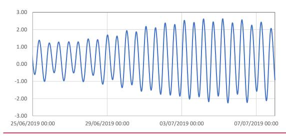
Figure 54. Tidal water levels (m ODN) at the existing outfall location
