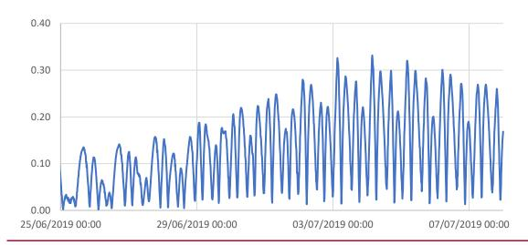
Figure 65. Current speeds (m/s) at the existing outfall location
