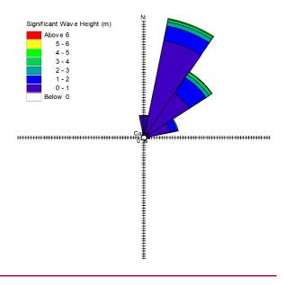
Figure 76. Nearshore wave rose (direction from °N) for Tees Bay - Oct to Dec 2003 (source: ABPmer (2004))
