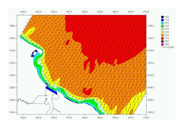
Figure 87. Wave height contours and direction vectors for 1 in 10-year waves (source: ABPmer (2004))
