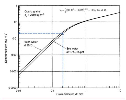
Figure 98. Estimation of settling velocity for medium sand (source: Soulsby (1997))
